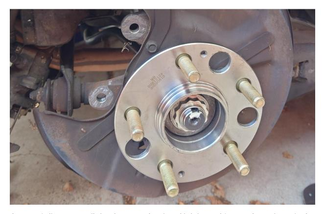
Torque the rear spindle nut to 140 lb ft and use a punch or large bladed screwdriver or other tool to stake the nut into place. Ensure the tangs of the stake are bent into the keyway on the spindle to ensure their retainment once covered.
