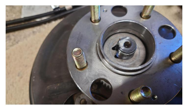
With the safety washer in place, locate the new 12-point nut included with your kit, and thread it on by hand. This too should thread easily into place. If it does not, DO NOT force it on with a tool. Remove the nut, check your threads, and retry. Should you cross thread the nuts you again risk premature failure and probable damage and/or injury to yourself and/or others.
