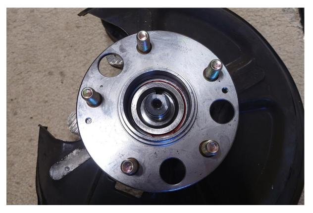
Once your hub is in place, locate your OEM Honda safety washer, and slide it onto the spindle – noting the tab slides into the keyway at the 12 o'clock position on the spindle.
