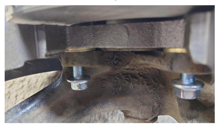
Torque to 80 lb ft. Use of medium strength thread locker is optional on these four bolts.
