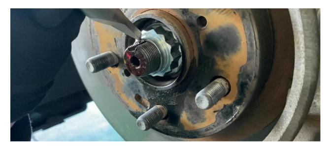
Locate your new rear brake rotor, clean thoroughly with aerosol brake clean (or a similar degreasing agent), and slide over the wheel study onto the rear hub.
