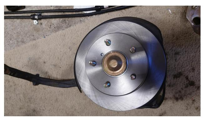
At this point we recommend using one of the previously set aside lug nuts to hold the rotor in place, as there is no rotor retaining screw for this application.
