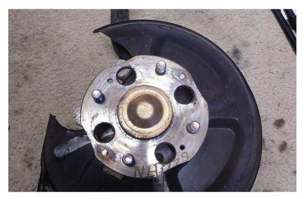
With the dust cover removed you will see the rear hub nut. Remove the nut with a 32mm socket and discard it. We HIGHLY recommend the use of an impact tool to aid in the removal of these nuts.
