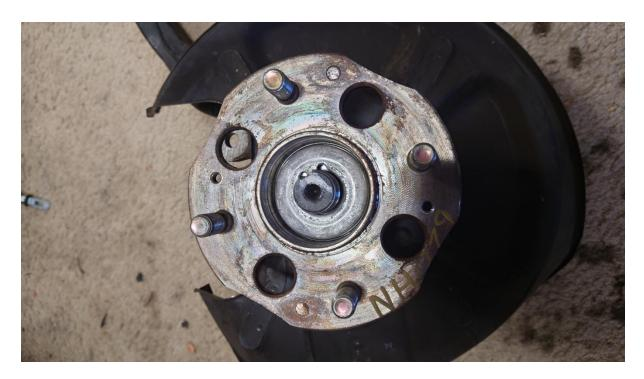
With the safety washer removed, the hub should slide off the spindle. Again to note, this may prove difficult depending on vehicle history, so work accordingly. However DO NOT damage the spindle surface with the tool you choose as this will lead to premature bearing failure and probable injury and/or damage to you and/or others.
