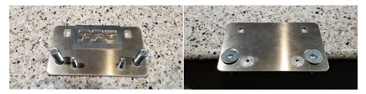
Flip the plate emblem side up, and slide the front holes in the shifter over the hardware.
