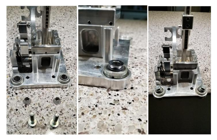
Take your assembly to your car, start the threads on the front 8mm x 30mm bolts in the forward plate, and then start the threads on each of the rearward 8mm x 40mm bolts. Once the threads are started, we recommend tightening each corner down about 7mm, then moving to another corner – to ensure an even compression of the assembly and tightening of the hardware.
