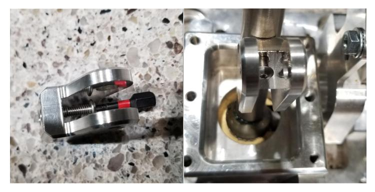
Tighten down the machine screws fully to seat the bracket against the shift lever. Once the bracket is attached to the shifter, insert your cable into the bracket, and then install the bolt with the sleeve. Only once final assembly tightened, add the serrated flange nut to the assembly and also final assembly tighten.
