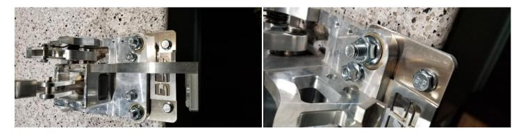
Tighten down the front two bolts, and tighten down your rear two mounting bolts to your car's tunnel. Once secure, tighten down the 12mm nuts as tight as possible. Remove the forward two 8mm x 30mm mounting bolts from your car's tunnel, and remove your rear two mounting bolts. Take the entire assembly to your workspace and tighten down the 8mm nuts and 12mm nuts (final installation).
